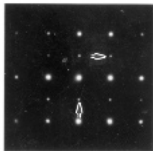
Figure 6 The transmission electron micrograph of the ternary phase (B2) present in the rapidly solidified (splat-quenched) Ti-25Al-25Nb alloy showing thermal APBs along with a SADP obtained from the B2 phase.
